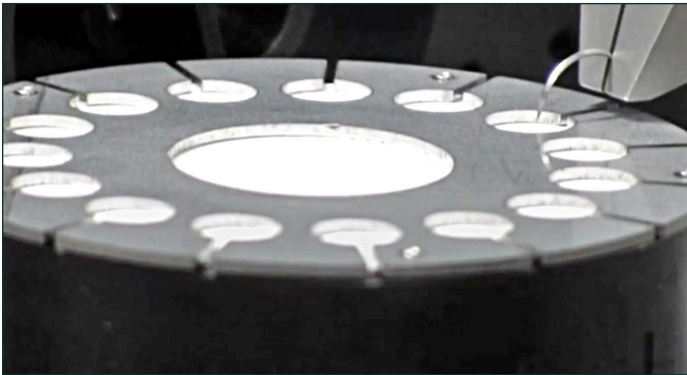
Penetration testing per ASTM International F3014-14 Standard.
