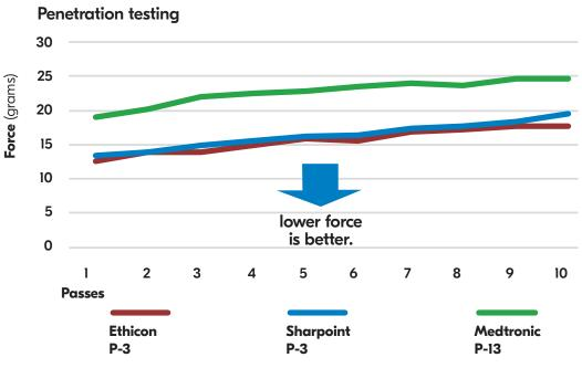
Penetration testing quantifies the force required for a needle to pass through a medium multiple times. 10 passes per needle. Performed by Acculine Engineering; an independent testing facility in Waterbury CT.
