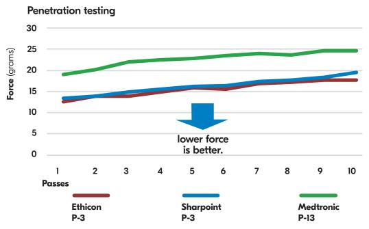
Penetration testing quantifies the force required for a needle to pass through a medium multiple times.
